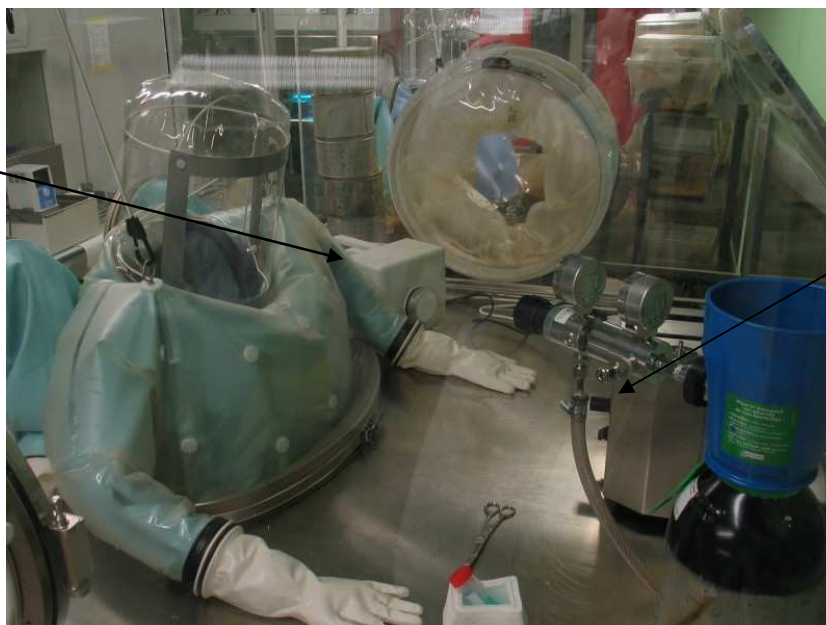
Fig. WP5-3: Another view of the half-suite isolator with the aerosol nebulizer and air sampler installed
