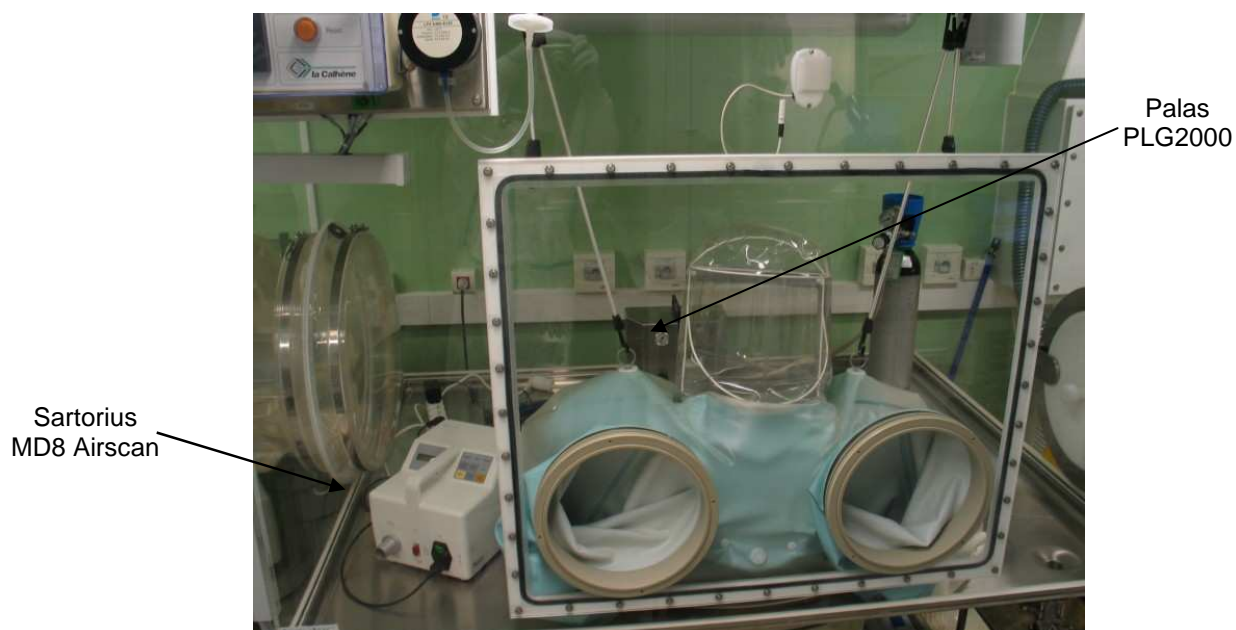
Fig.WP5-2: Picture of the half-suite isolator with the aerosol nebulizer and air sampler installed
